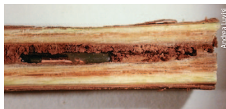
An RFID microchip was placed longitudinally in a grapevine. Plant-specific data can be used for certifying stock, monitoring pests and mapping vineyards.
