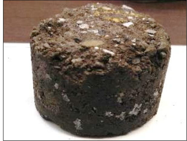
Figure 5.7: ITS specimen with edge damage after cutting.
