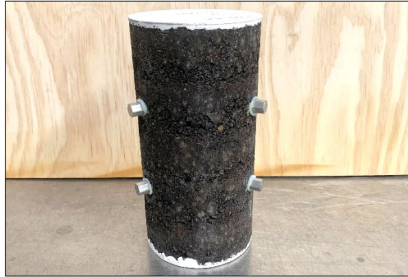
Figure 3.4: Gypsum caps after removing tape from both ends.
