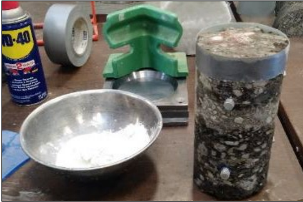
Figure 3.3: Preparing to apply gypsum cap.
