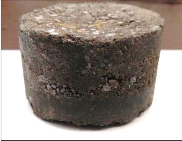
Figure 5.6: ITS specimen with no damage after cutting.
