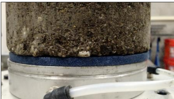
Figure 3.1: Inconsistent specimen ends leading to poor contact.
