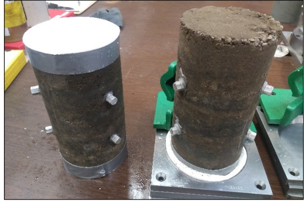
Figure 5.4: Compacted specimen being capped with gypsum.
