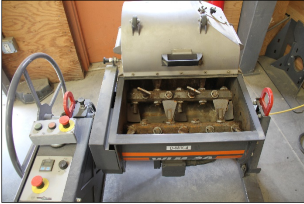
Figure 5.3: Paddle mixer used to mix material, cement, and water.
