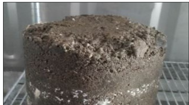
Figure 3.2: Broken edges due to pull out of recompressed faces.
