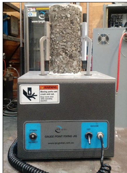
Figure 3.5: Modified gauge point jig with gauge point holders for 200×100 mm specimens.
