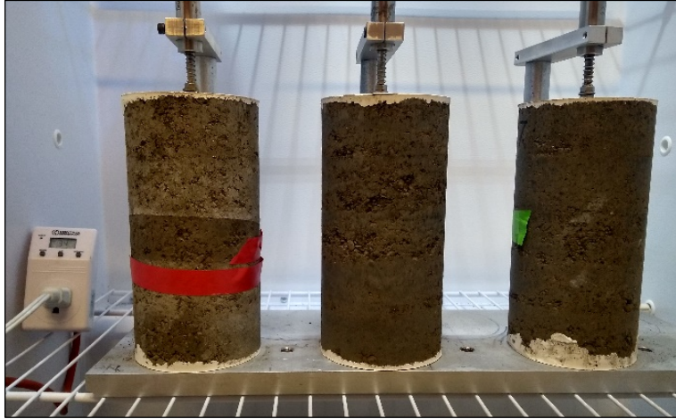
Figure 5.8: Free-drying shrinkage test setup.
