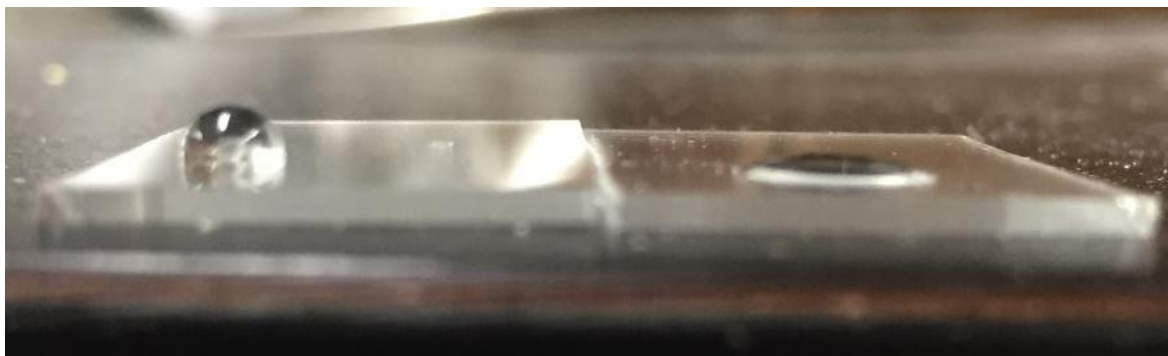
Figure C3. Images showing a water droplet on perfluoroalkyl functionalized (left) and bare (right) glass substrates. Contact angle for the coated surface was measured to be approximately 115°.
