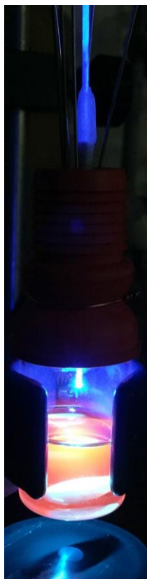
Figure A12: Photograph of benchtop reaction of (i) using a 470 nm fiber-coupled LED.
