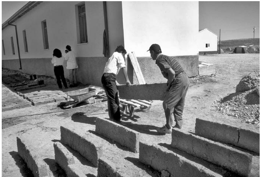
Figure 22.6. Brick manufacture: mud bricks drying.
