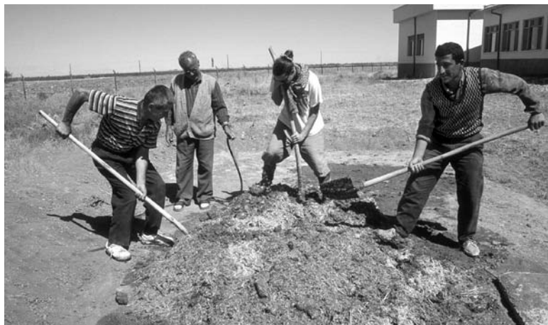
Figure 22.2. Brick manufacture: adding the straw and chaff.
