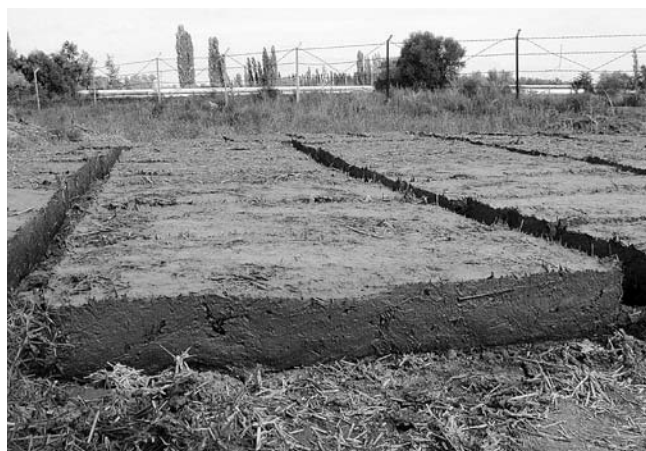
Figure 22.3. Brick manufacture: laying bricks on the ground.
