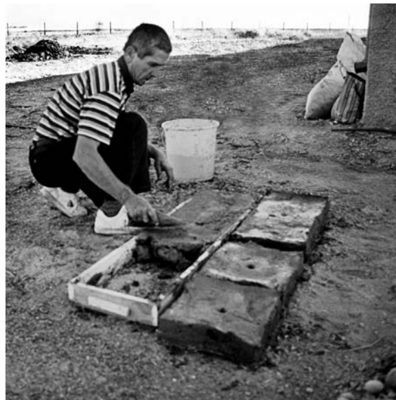
Figure 22.4. Brick manufacture: pouring the mix in the molds.
