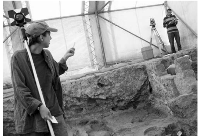
Figure 2.9. Laura Steele and Vuk Trifković using the EDM to document measurements on a field drawing in 2000.
