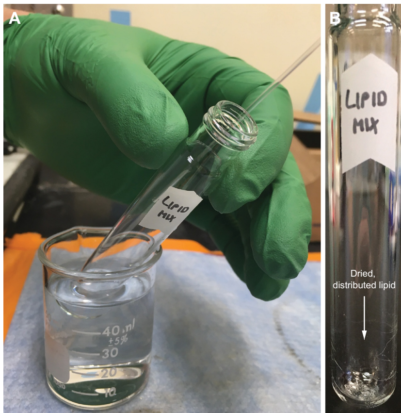
Fig. 2 (A) Set up for removing solvent from lipids. (B) Properly dried lipid is distributed in an even thin film at the base of the glass tube.
