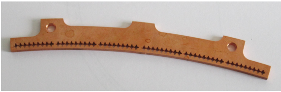
Fig. 15 Fiber holder produced with wire erosion. Note the pattern of diagonally aligned square holes. One holder covers an angular range of 23.5^\circ .
