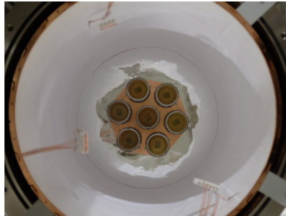
Fig. 11 Bottom PMT plate with 7 PMTs and copper cylinder. Plate and cylinder are covered by wavelength shifting Tetratex ® foil soaked in TPB [23].
