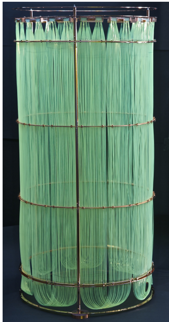
Fig. 14 The fiber curtain: height \sim 1 m, diameter \sim 0.5 m, 405 fibers read out on both ends by 90 SiPMs.
