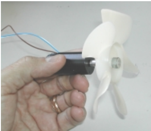
Figure 2: Miniature airflow turbine.
