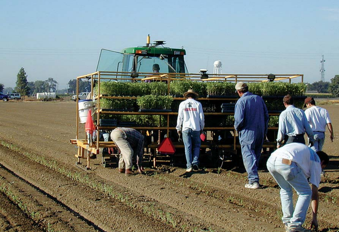
Ultraprecise global positioning systems (GPS) are now available that can guide tractors at high speeds in agricultural fields, running to within inches of plants with very little damage. Above, at UC Davis, tomato seedlings are transplanted using an autoguidance system. The GPS unit is on top of the tractor cab. Left, drip tape is installed at the same time.
