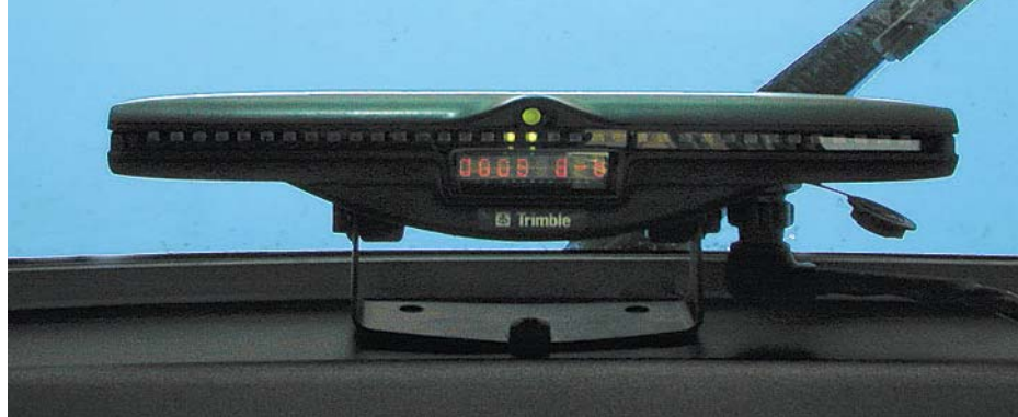
Left , a fertilizer shank is used in deep tillage operations to determine the ability of the autoguidance tractor and implement to stay clear of buried drip-tape. Above , on the light bar in the tractor cab, a green LED in the center indicates that the GPS unit is on track.
