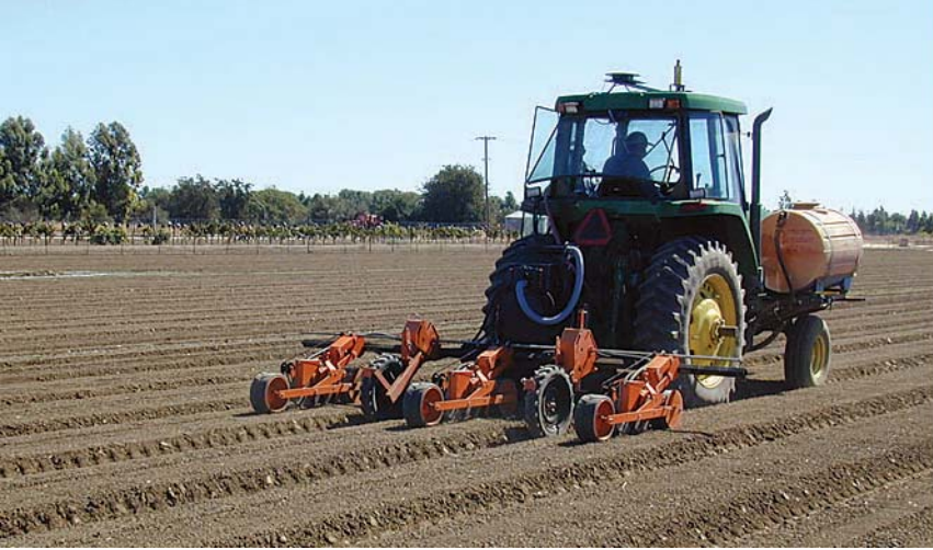
Processing tomato seeds are planted using an autoguidance system. In two trials, total plant damage was 2% and zero when the autoguided cultivator was operated at 7 miles per hour and 2 inches from the plant line.
