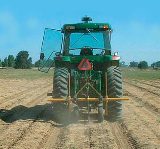
Left , a fertilizer shank is used in deep tillage operations to determine the ability of the autoguidance tractor and implement to stay clear of buried drip-tape. Above , on the light bar in the tractor cab, a green LED in the center indicates that the GPS unit is on track.
