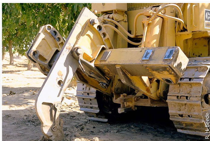
Figure 15. Deep-ripping implements can be used to destroy old burrow systems.
