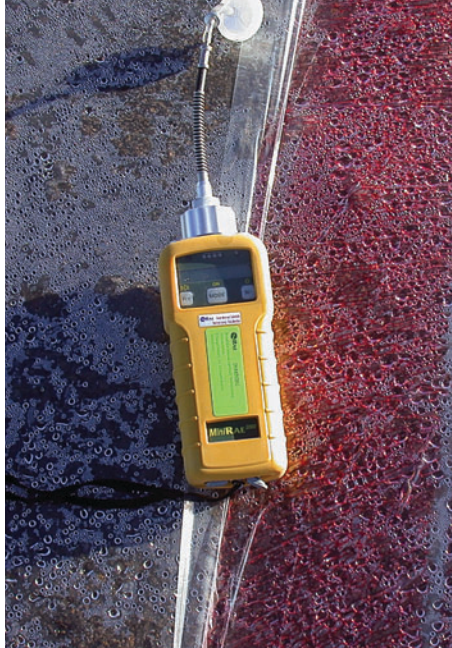
A meter was used to measure volatile organic compounds (VOCs), which can react with nitrogen oxides to form air pollutants.
